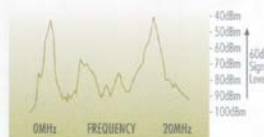
Figure 3 Typical HF spectrum occupancy.
